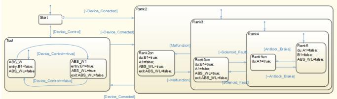
Fig. 3 Developed controller for the desired system on Stateflow® block diagram, for ABS Indicator Lamp.
