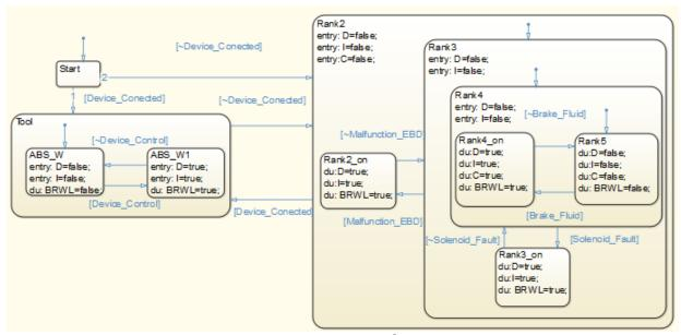
Fig. 4 Developed controller for the desired system on Stateflow® block diagram for Brake Warning Light.
