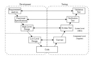
Fig. 1. The workflow of V-model for automotive embedded systems.
