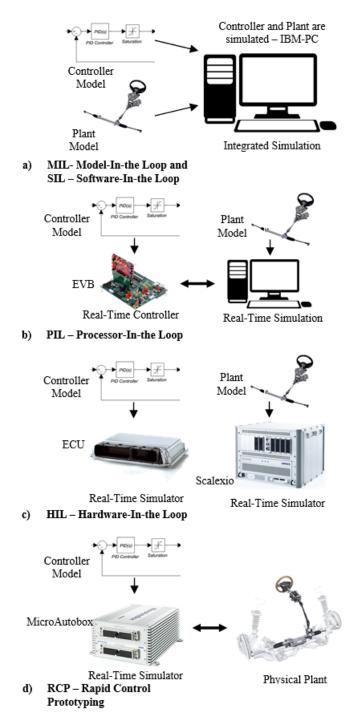
Fig. 2. Application categories of MIL, SIL, PIL, HIL and RCP.
