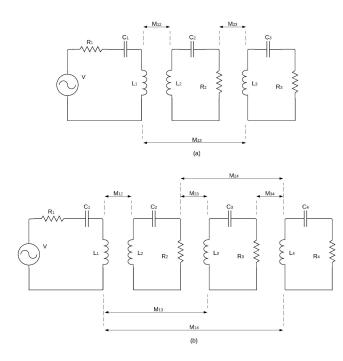
Fig. 1. Wireless power transfer system (a) with 3 coils (b) with 4 coils. The leftmost circuits are the primaries or the excitement. The rightmost circuits are connected to the load, represented by R3 or R4, respectively. The intermediate circuits are for coupling and energy transfer and must have minimum resistance values. (Modified from [36])
