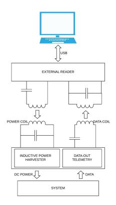
Fig. 2. Block diagram of a wireless system for an implantable medical device.
